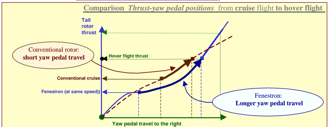
With a Fenestron, when changing from **cruise flight to hover flight**, be prepared for a **significant movement of the foot to the right**.
