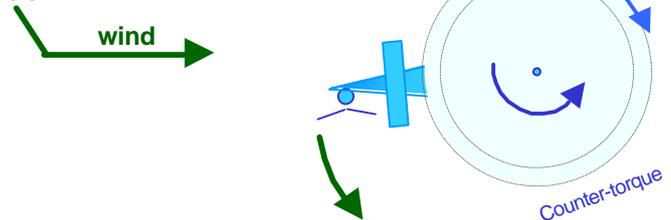
In a quick leftward rotation, if the Pilot attempts to counteract this rotation by applying the RH yaw pedal up to a position corresponding to that of hover flight, the aircraft will not decelerate significantly!
